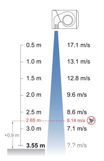
According to standard NSF-37-2012, the maximum installation height is the speed profile point at 8.14m/s plus 0.9m. So FLY KBB can be used until 2.65m+0.9m=3.55m.
